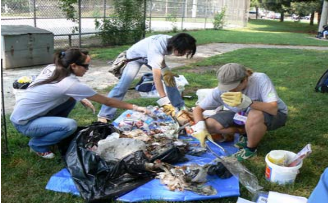
Photo 9: Waste audit methods. Sorting waste into categories on a tarp using tongs.
